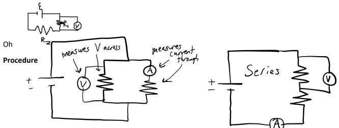
You will want at least one circuit with 3 resistors in series and one with 3 circuits in parallel. Circuit diagrams show examples for both (series on the right, parallel on the left) with 2 resistors each. Measure the voltage and current across each resistor and filling in the tables below.
